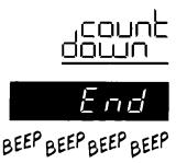
When the cooking time ends, "End" will show on the Display and 4 beeps will sound. You can stop the beeping by opening the door or by touching CANCEL.) "End" will remain on the Display and a beep will sound every 60 seconds (to remind you that food is left in the oven) until the door is opened or CANCEL is touched. The Display will then show the time of day.
